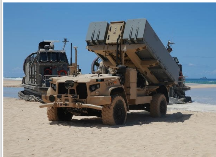
A Navy Marine Expeditionary Ship Interdiction System launcher deploys into position aboard Pacific Missile Range Facility Barking Sands, Hawaii. During the training, a Marine Corps fires expeditionary advanced base sensed, located, identified and struck a target ship at sea, which required more than 100 nautical miles of missile flight (U.S. Marine Corps photo by Maj. Nick Mannweiler, released).
